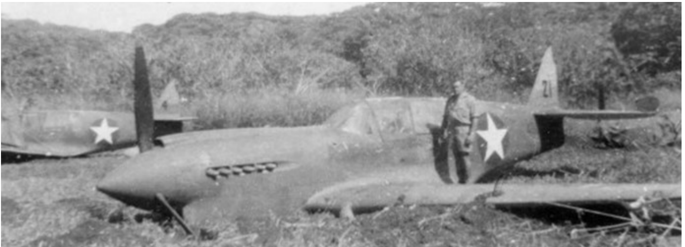
A few of the unserviceable 68 th FS aircraft left were used as decoys on the surrounds of the base, buried with undercarriage extended and rudderless. Odd yes, with P-40E-1 41-25139/ET463 #21 later repaired as NZ3095. [Buz Album Collection].
