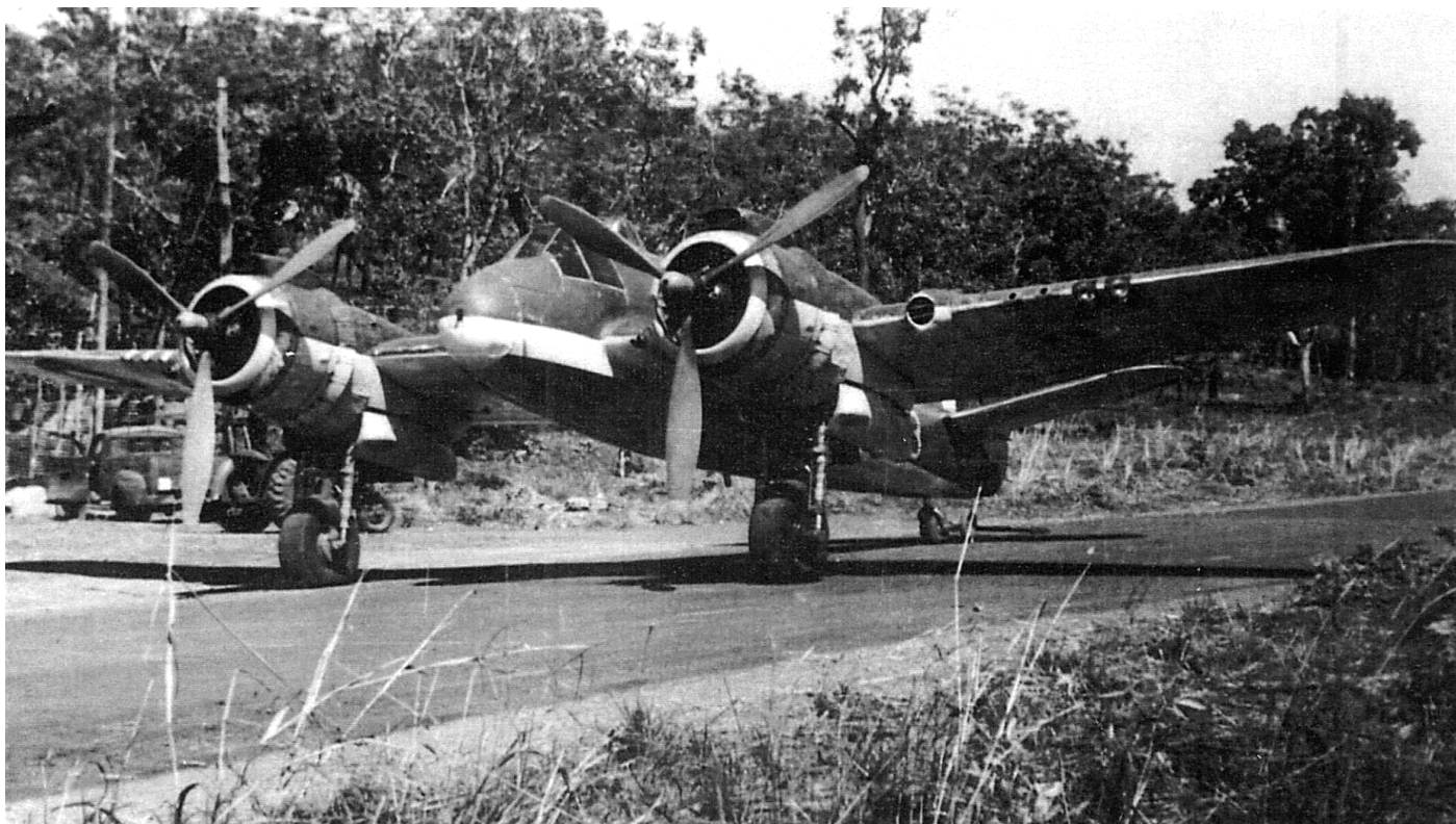
I reckon this is A19-169/EH-B. Of the three British built Beaufighters operated by 31SQN with the individual identification letter "B", only A19-169 had the 12° dihedral horizontal stabilizer. The positioning of the demarcation between the upper camouflage (original British Temperate Sea Scheme or perhaps Foliage Green and Dark Earth?) and the lower camouflage (RAAF Sky Blue) is unusual and seems superficially similar to the scheme originally intended for RAAF Mosquito's. [Image courtesy of 31 Squadron Beaufighter Association].
