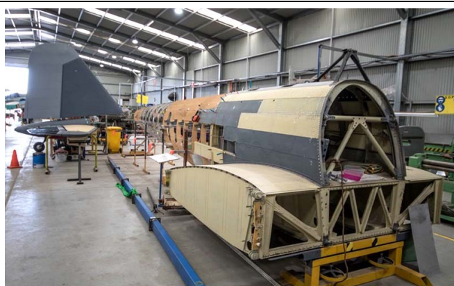
Centre wing section was mated with the fuselage in 2015
