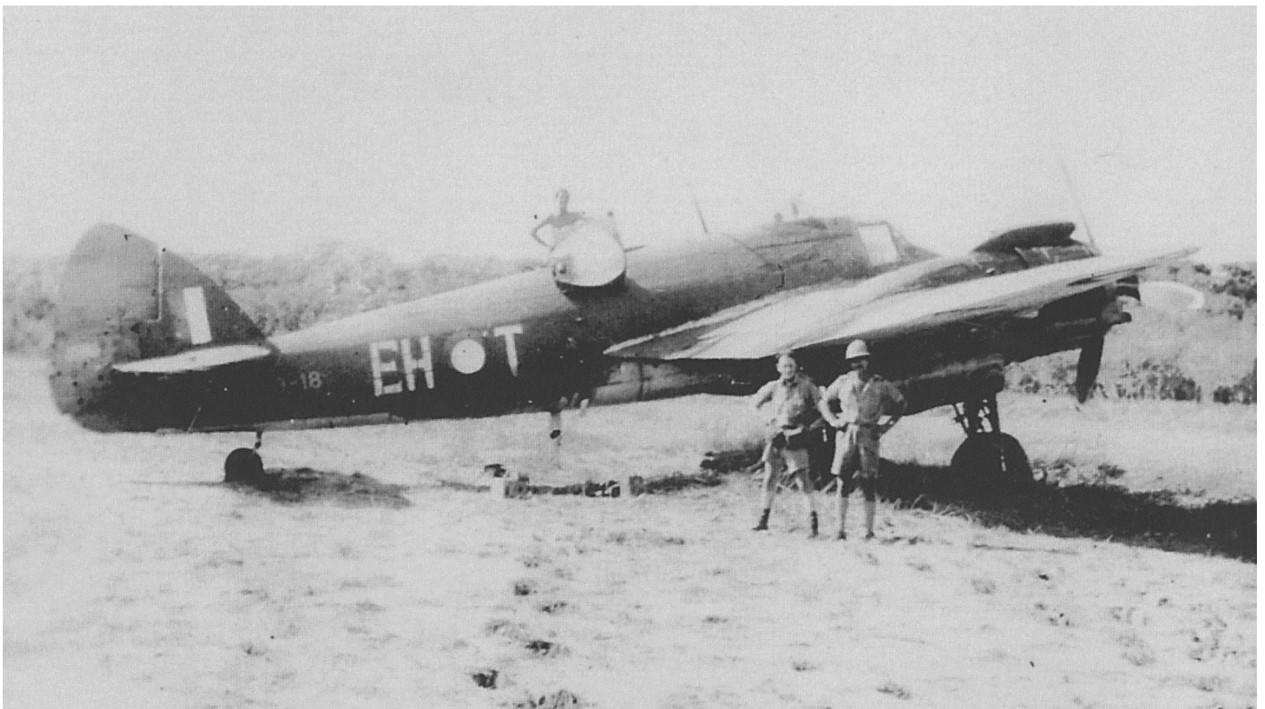
The flat horizontal stabilisers are illustrated here by 31SQN's A19-18/EH-T as it sits, dripping oil, on a convenient piece of flat, unobstructed ground, a considerable distance from the nearest airfield. The date was August 18 th , 1943, and A19-18 had been engaged on a convoy escort. During the course of that job and whilst at (evidently) low level over the water the oil cooler of the starboard engine was ruptured (presumably by a shell casing) which had, no doubt, bounced off the water and hit it during the course of "test firing". The starboard engine was run dry due to engine oil being vented overboard and the engine was later assessed as being damaged beyond repair. Aside from that minor detail, there was no damage to the aircraft or crew. They were located by another of the squadron's machines which landed next to them and took them back to base. The aircraft was later repaired by 4RSU and returned to 31SQN on September, 21 st . One wonders how the explanation was received by the Boss. [Image courtesy of 31 Squadron Beaufighter Association].
